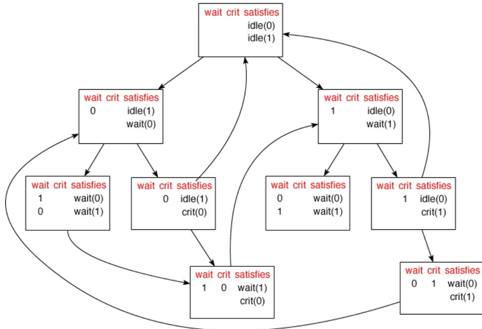
Fig. 4. The Kripke model derived from MUTEX for two processes after its transformation performed by drawK
